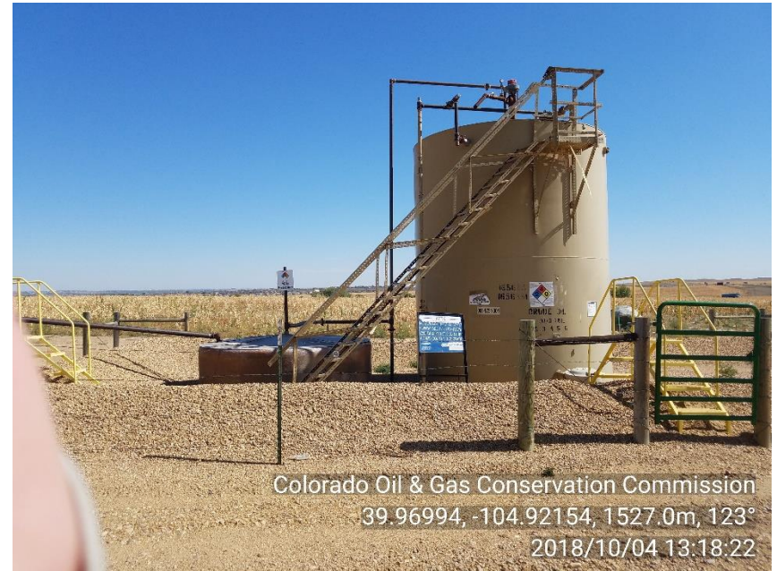
PHOTO 2: TANK BATTERY
