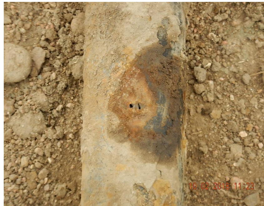
Close up view of a corrosion hole found on the failed section of flowline associated with the Amoco-Charter-Schneider 12A well (API 123-09038)
