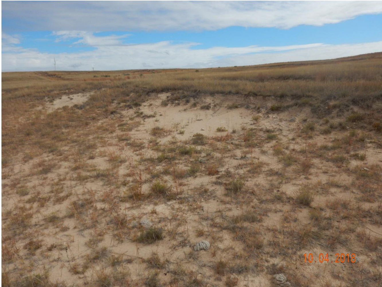
Photo 1: Photo taken from the southeast end of the location, facing northeast. Previous inspections documented that areas of the east end of the location and access road have not achieved a uniform desirable perennial vegetative cover, and stormwater has caused erosion degradation. Inspections required operator to perform reclamation and stormwater management. Photo shows no management activities per the CAs appear to have been conducted; location/access road has not been adequately contoured/graded and revegetated, sotrmwater has continued to cause erosion degradation.
