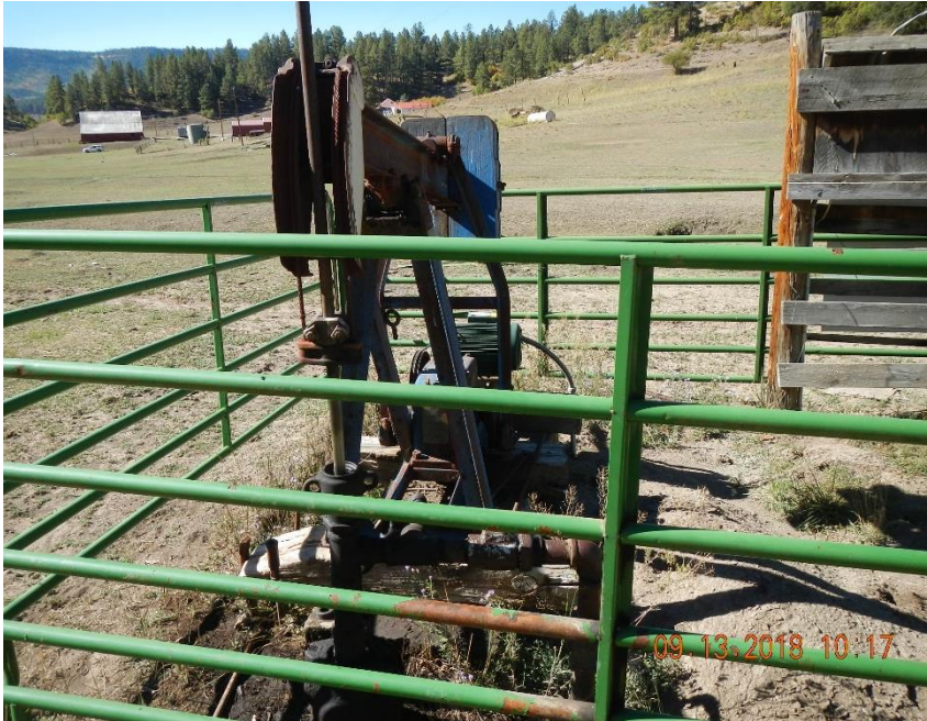
Fitzhugh #6 pump jack and well head. Stained soil surrounding well.
