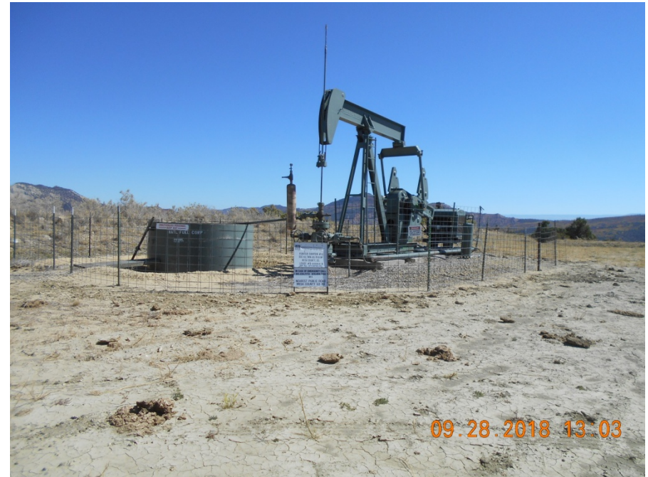
Wellhead with pump jack and produced water tank
