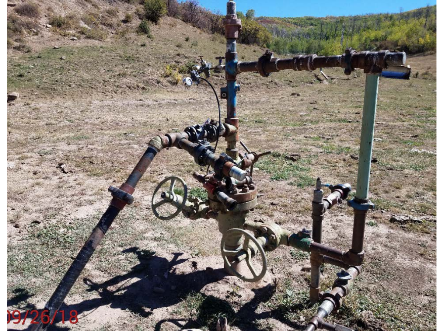
Location Photo #2, missing wellhead sign.
