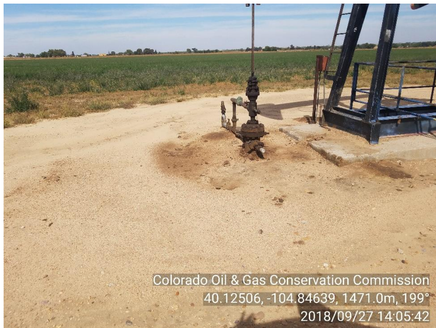
PHOTO 3: STAINED SOIL AROUND WELLHEAD
