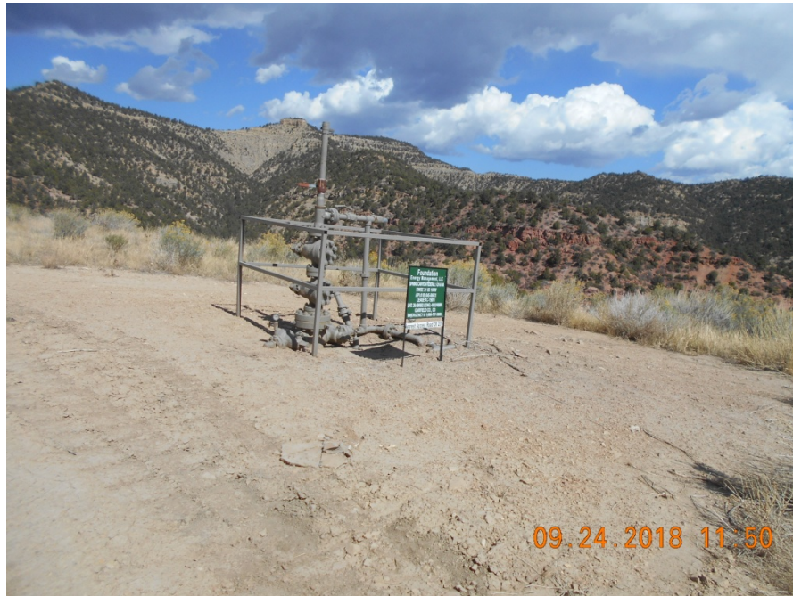
Wellhead with fencing and sign
