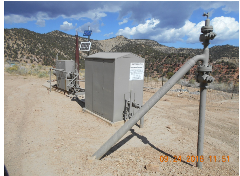
Separator and meter housing
