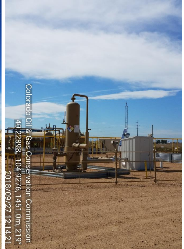
Photo 3 Vert Separator and GMR Shack
