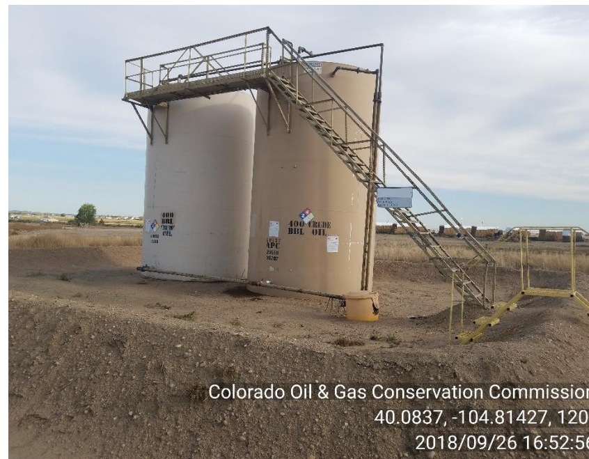
PHOTO 2: TANK BATTERY
