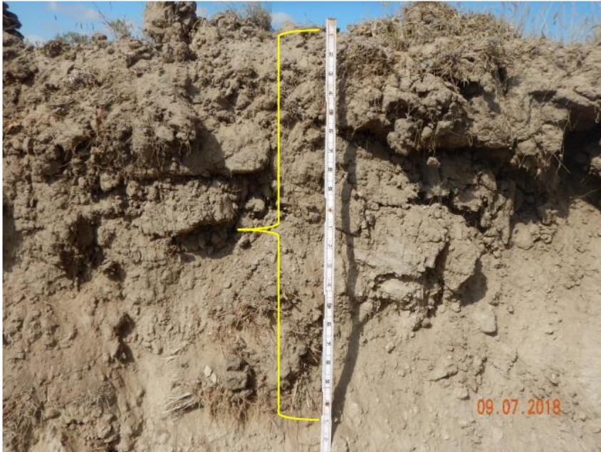
Photo 5: Continued from photo 4. Photo shows the topsoil horizon. Topsoil horizon appears to be ~2 feet in depth. 6 foot measuring stick for reference.
