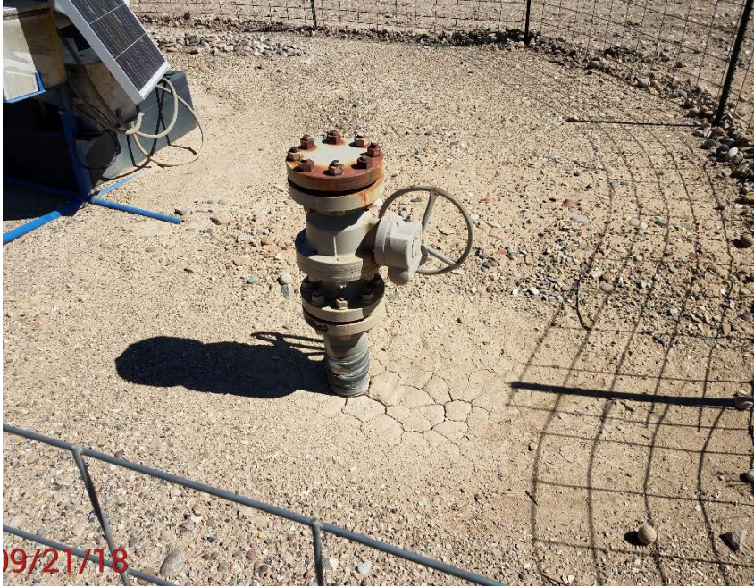
Location Photo #3, unmarked flow line riser.
