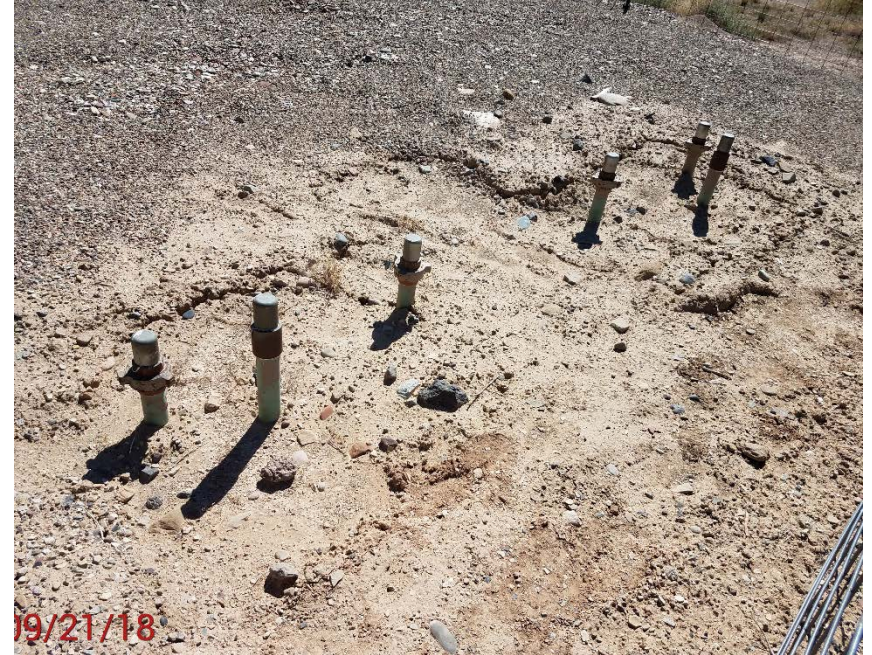
Location Photo #4, 6 unmarked flow line risers
