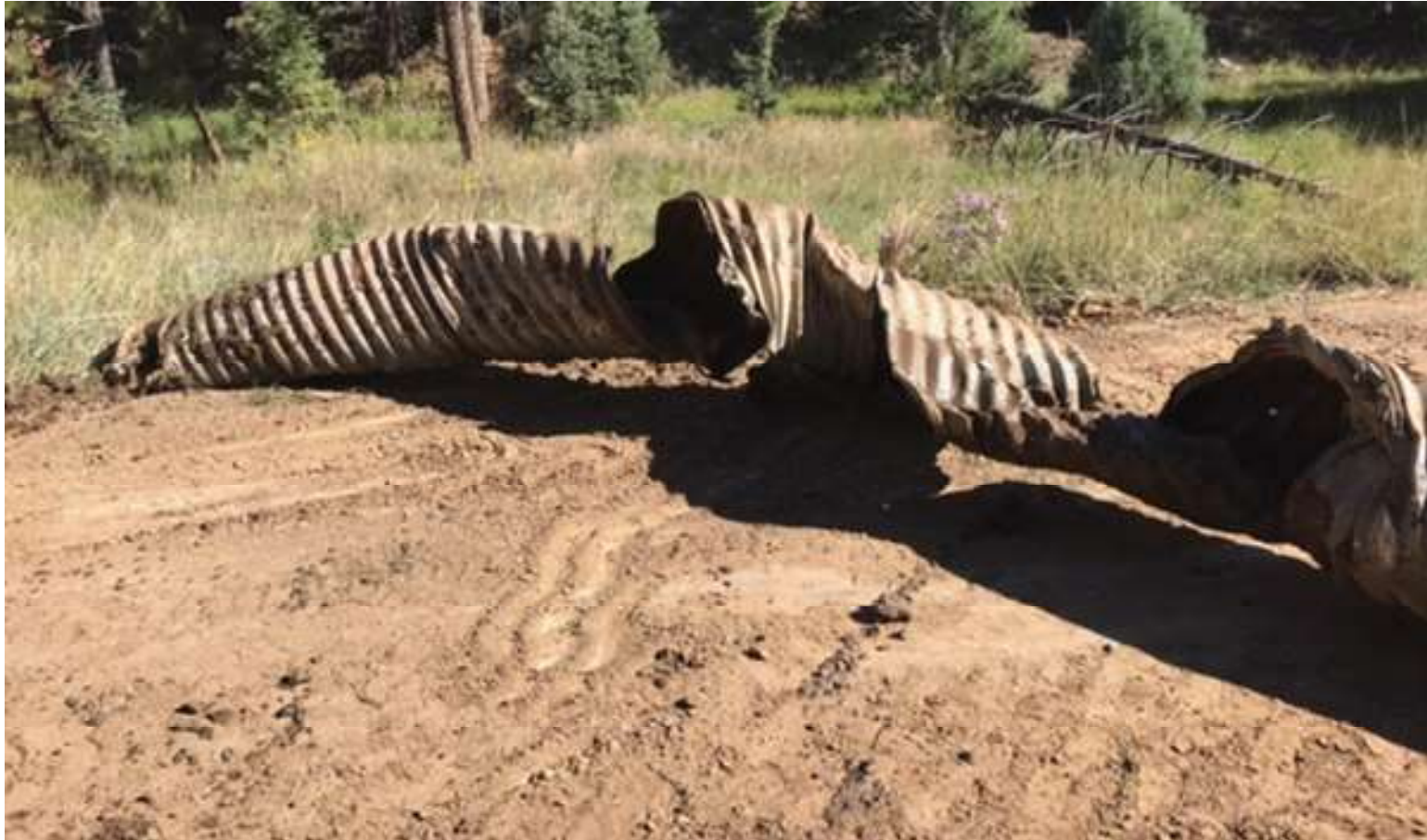
PHOTO 3: THE DAMAGED GALVANIZED CULVERT ON THE MAIN LEASE ROAD WAS REMOVED.
