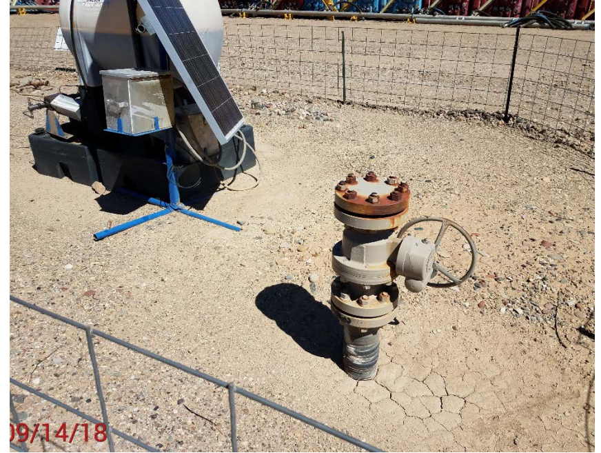
Location Photo #4, unmarked flowline riser
