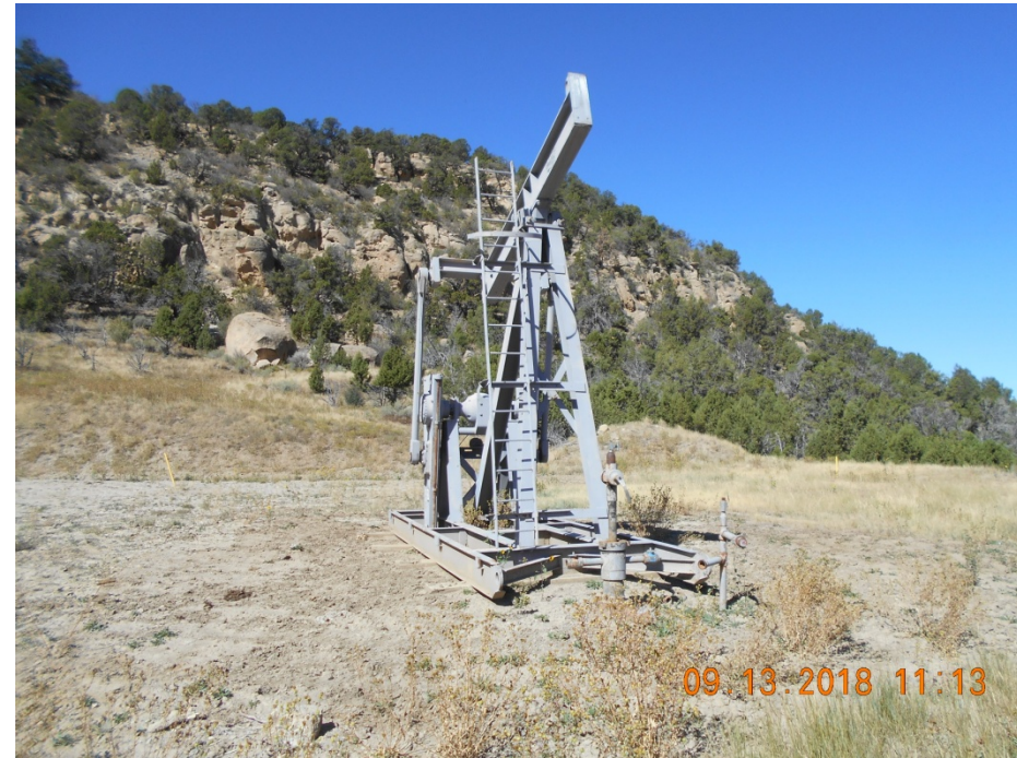
TA wellhead with unused pump jack
