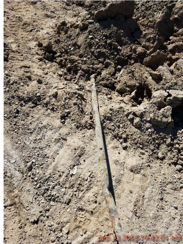
Photo 4 – Corrosion hole in removed dumpline.
