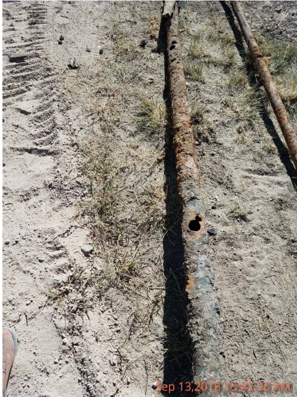
Photo 3 – One of several corroded dumphines.
