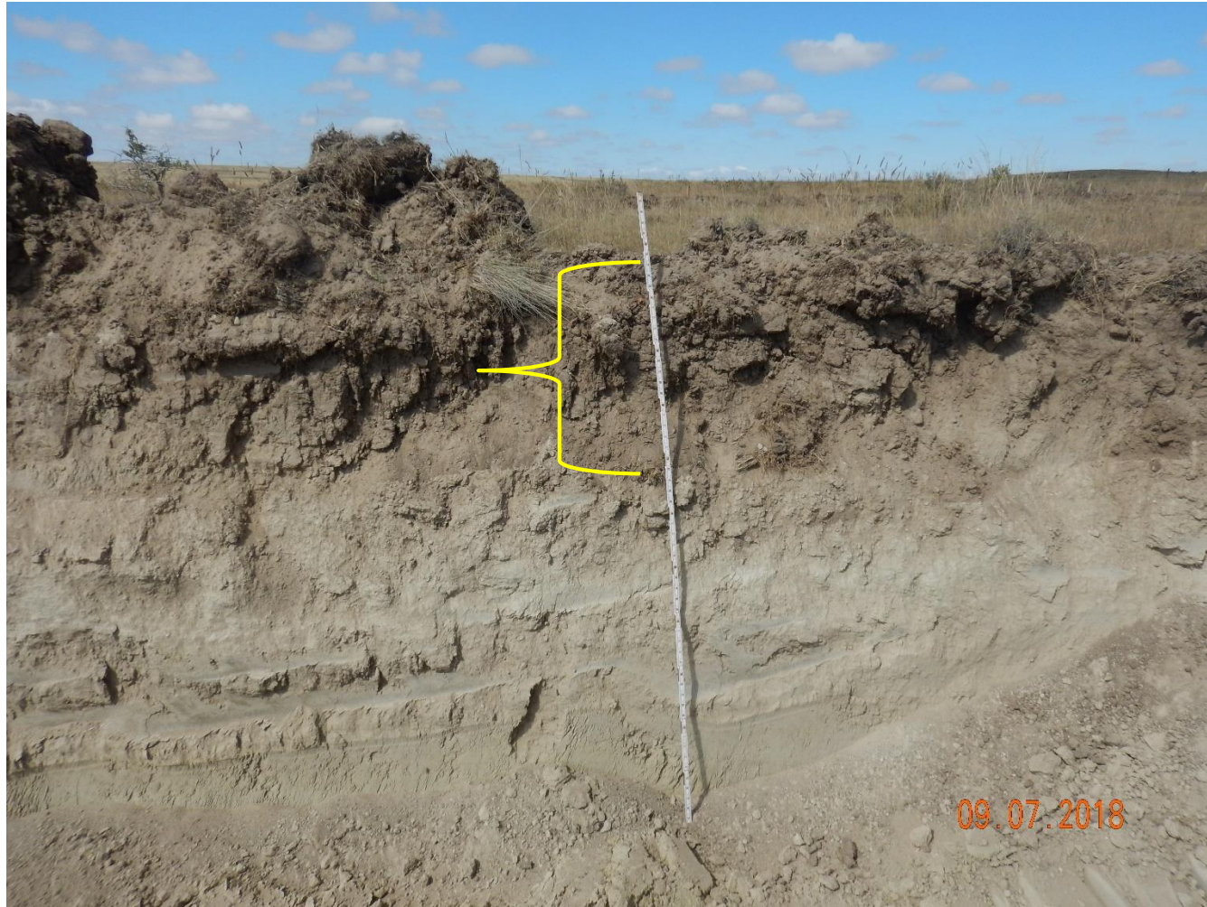
Photo 4: Photo taken from the northwest corner of the pad. Photo shows the topsoil horizon. Topsoil horizon appears to be ~2 feet in depth. 6 foot measuring stick for reference.
