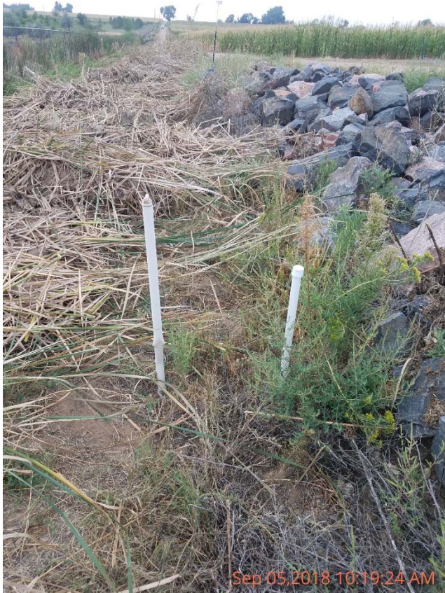
Photo 3 – Damaged monitoring well on east side of source area/adjacent ditch.
