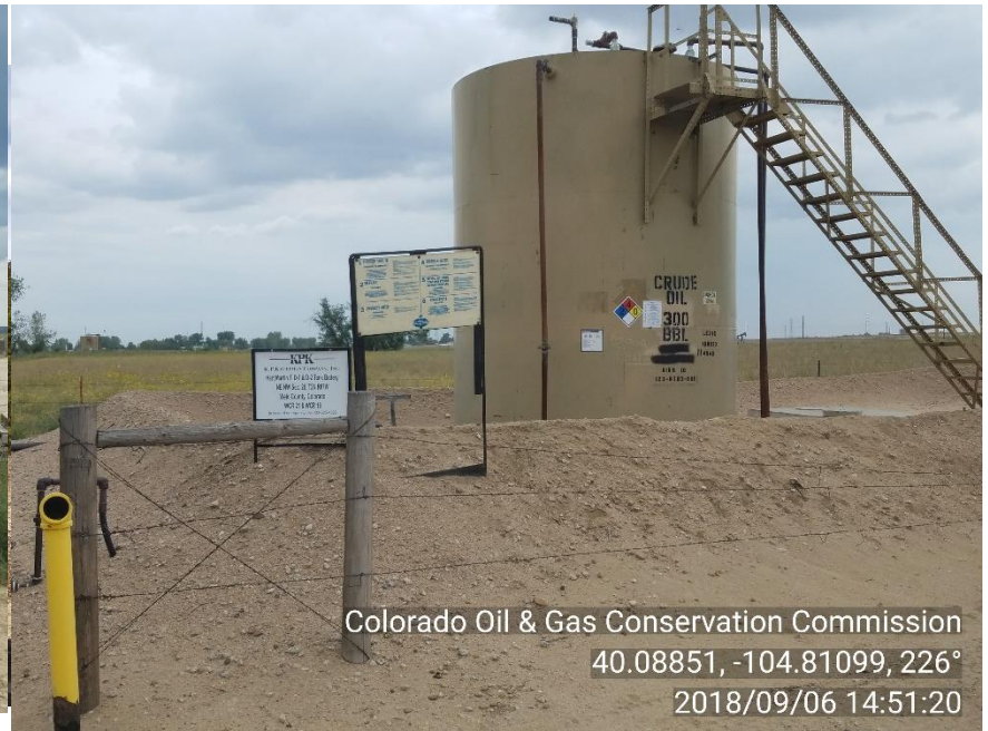
Photo 2. Tank battery/Unmarked unplugged riser
