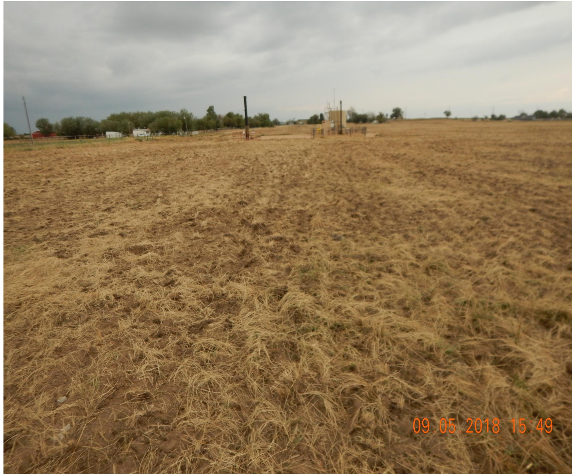
Photo 4. Reference photo taken west of the location, facing West. Photo illustrates little to no rock fragments of similar size or density were observed in reference areas. This indicates the Operator failed to remove gravel and perform compaction alleviation.
