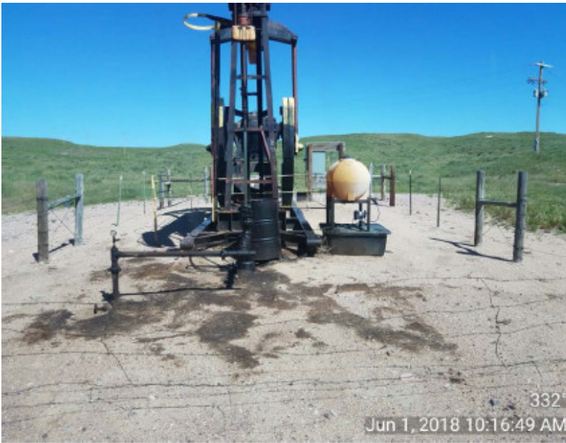
Photo #1 Moyer Unit 16-29 (API 05-123-07014) wellhead Stained soil From previous FIR
