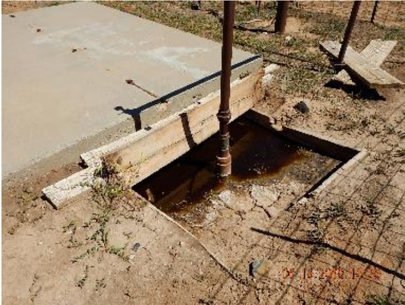
Photo 3: Wellhead cellar with standing fluids. Previous inspection.
