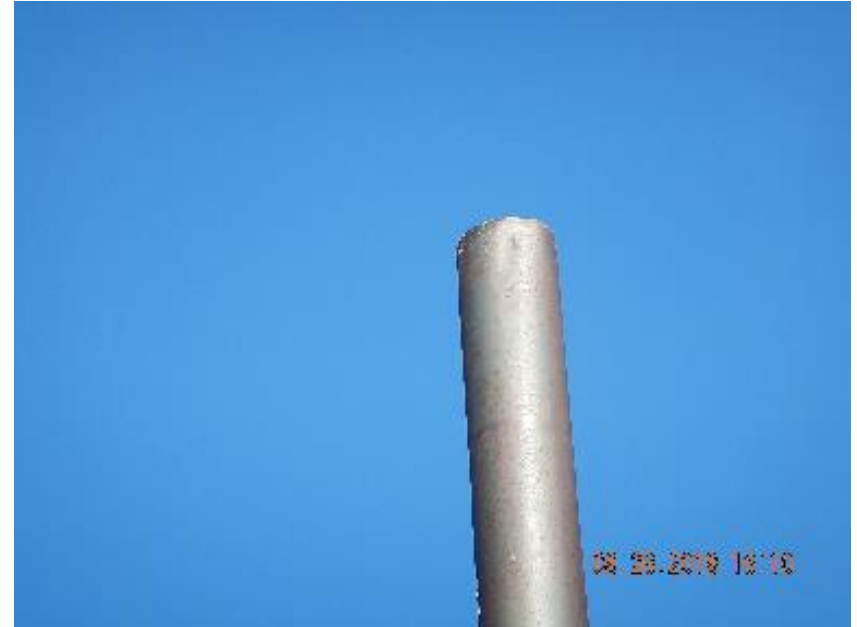
Photo 6: Stack at the Spargo #2 FG separator without bird screen.
