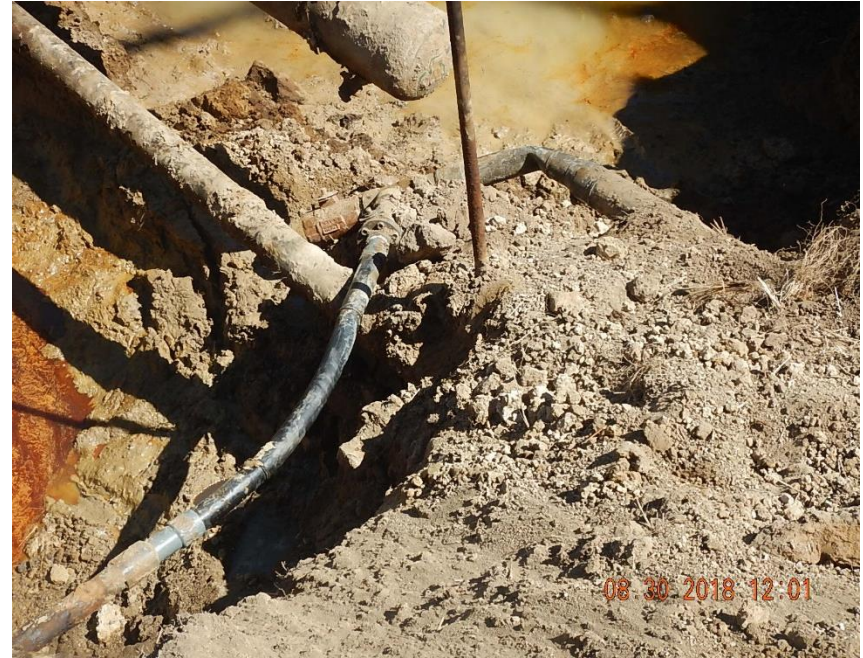
Closer view of the kink at the 2" to 4" transition of the off location poly flowline.
