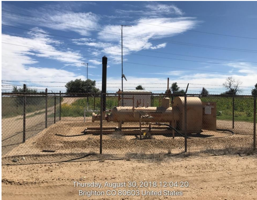
Photo#3 Separator and Gas Meter
