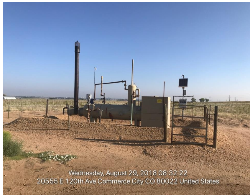
Photo#2 Separator and Automation RTU
