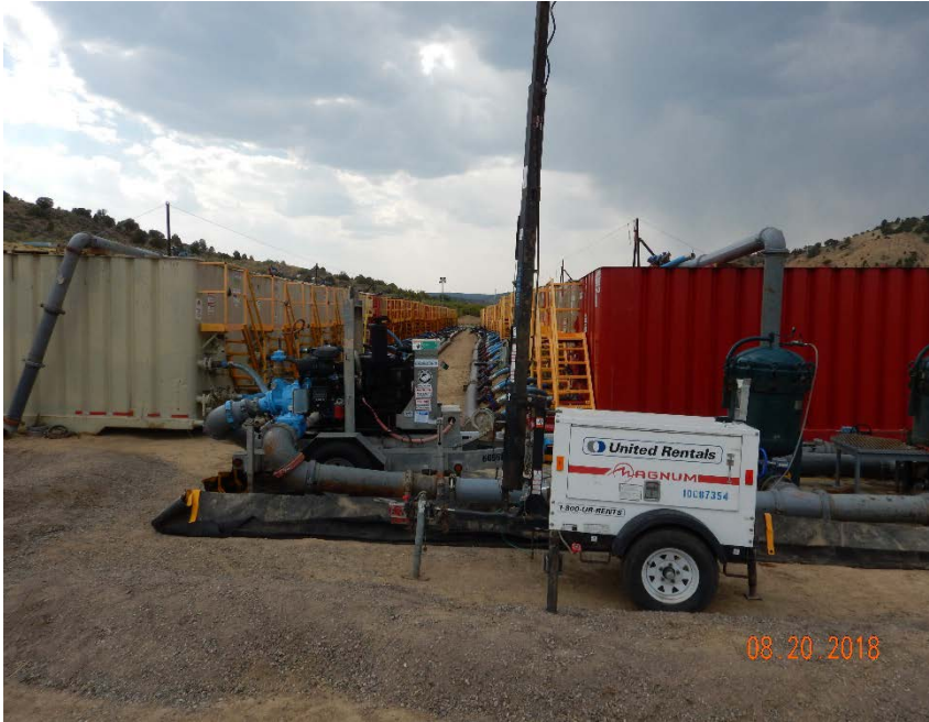
Photo #3 – Frac tanks are plumbed to support ongoing E&P operations. View of southern tanks, looking west.
