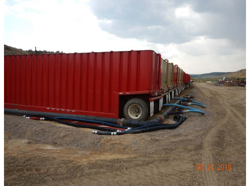
Photo #2 – View of bermed frac tanks lining south side of location, looking west.
