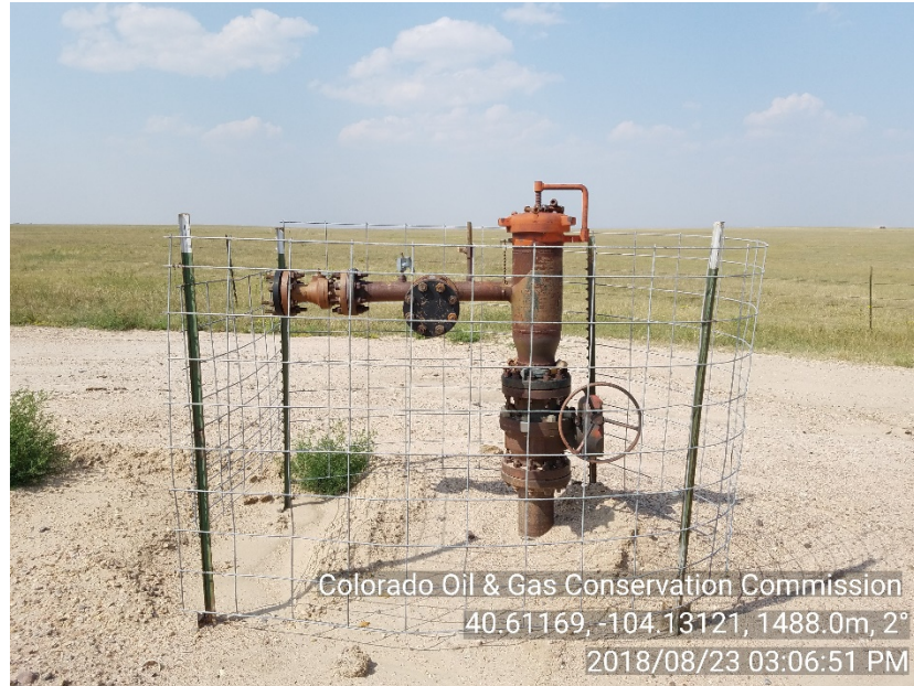
Photo # Hill 31-15-8, 31-9-11, 31-14-7 Remaining pig launcher
