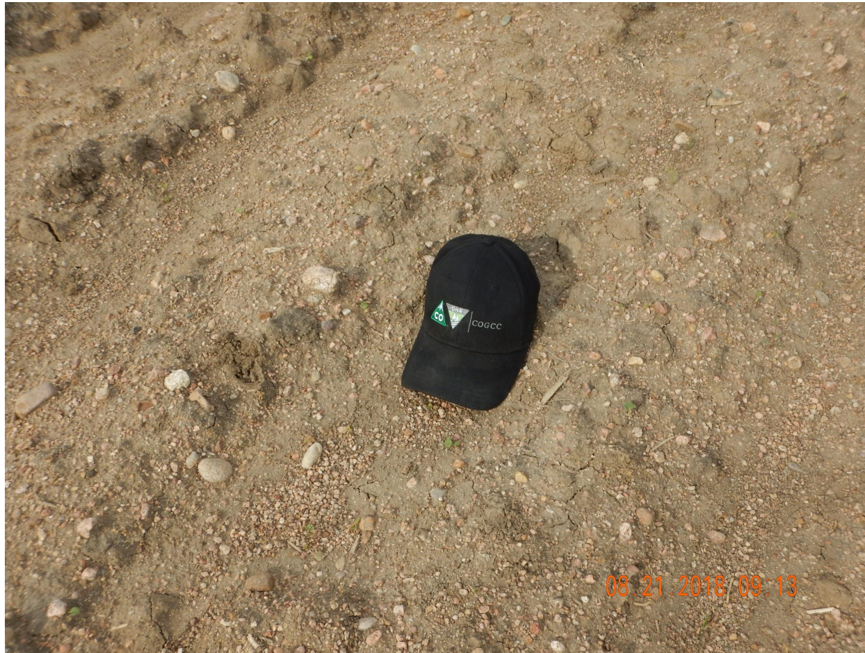
Photo 5. Photo taken from a portion of the excavated area. This area (orange line in first slide) does not appear to be soil material that is equivalent to reference area soils, as this soil material consisted of coarse rock fragments not observed in reference areas. Soil samples were collected for confirmation. Operator shall ensure all imported soil is the same or equivalent to that of reference area soils.
