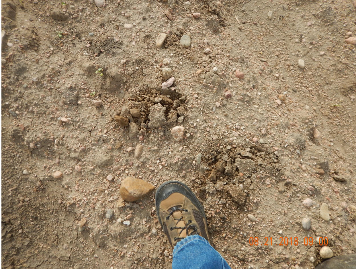
Photo 6. Photo taken from a portion of the excavated area. This area (orange line in first slide) does not appear to be soil material that is equivalent to reference area soils, as this soil material consisted of coarse rock fragments not observed in reference areas. Soil samples were collected for confirmation. Operator shall ensure all imported soil is the same or equivalent to that of reference area soils.
