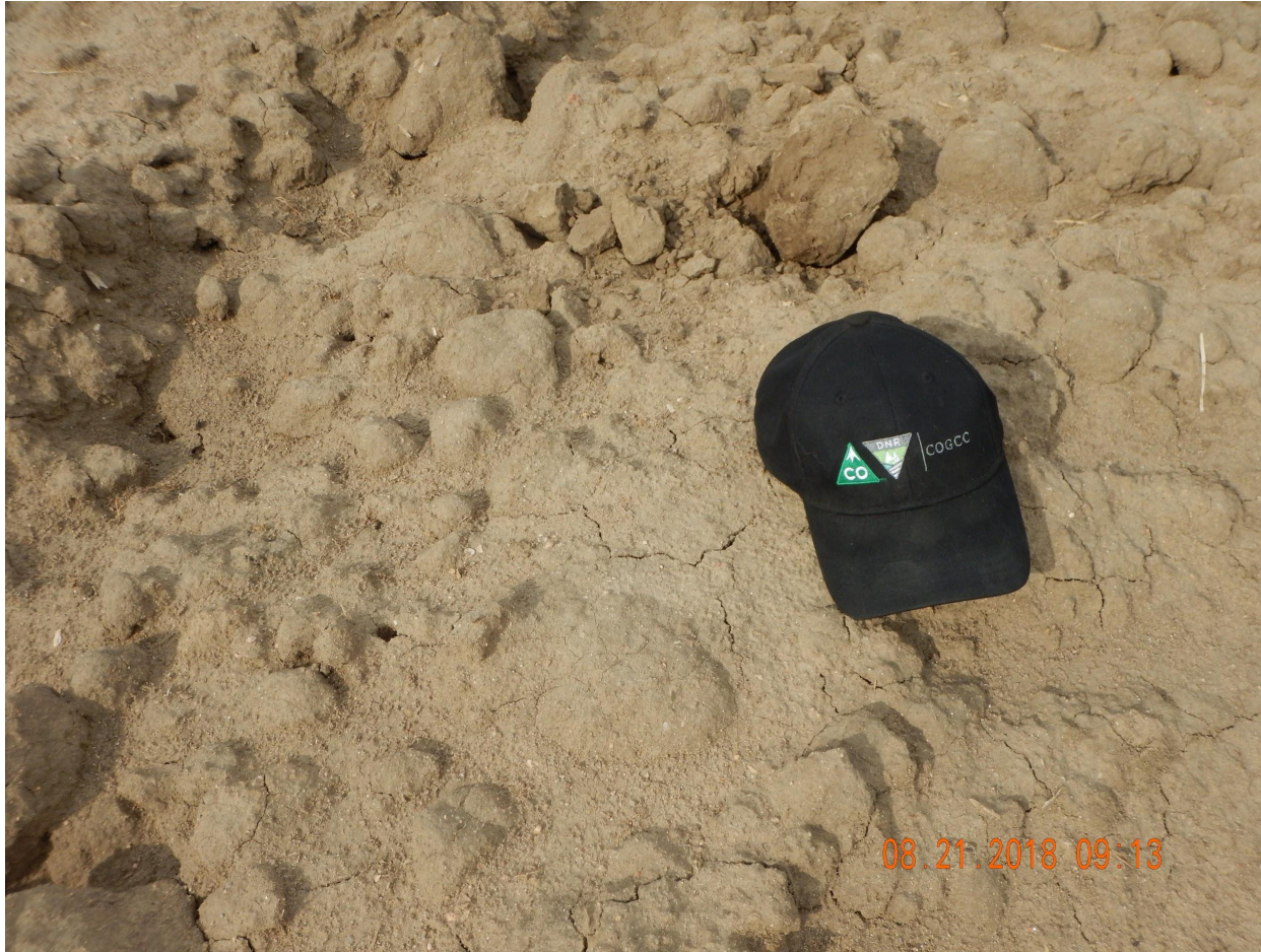
Photo 4. Photo taken from a portion of the excavated area. It is unclear whether or not this soil material is equivalent to reference area soils. Soil samples were collected for confirmation. Operator shall ensure all imported soil is the same or equivalent to that of reference area soils.
