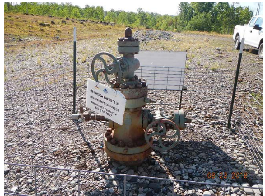
Photo 2. Wellhead is not connected to any production equipment.
