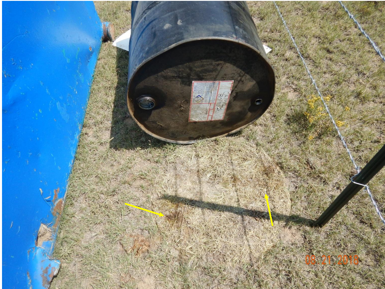
Photo 30: Continued from photo 29. Photo shows barrel was placed open on the soil surface. Photo shows contaminants on soil surface.
