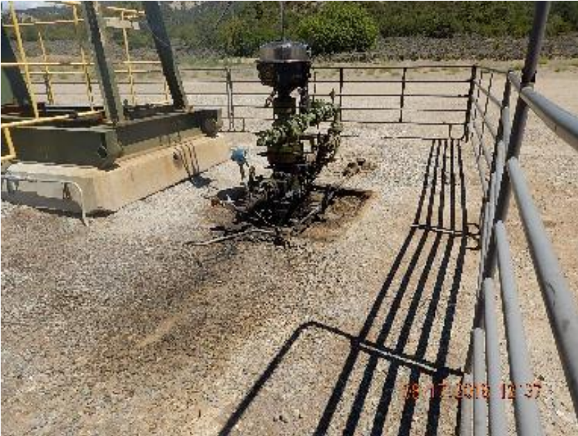
Photo 5: Impacted soil and gravel around base of wellhead.
