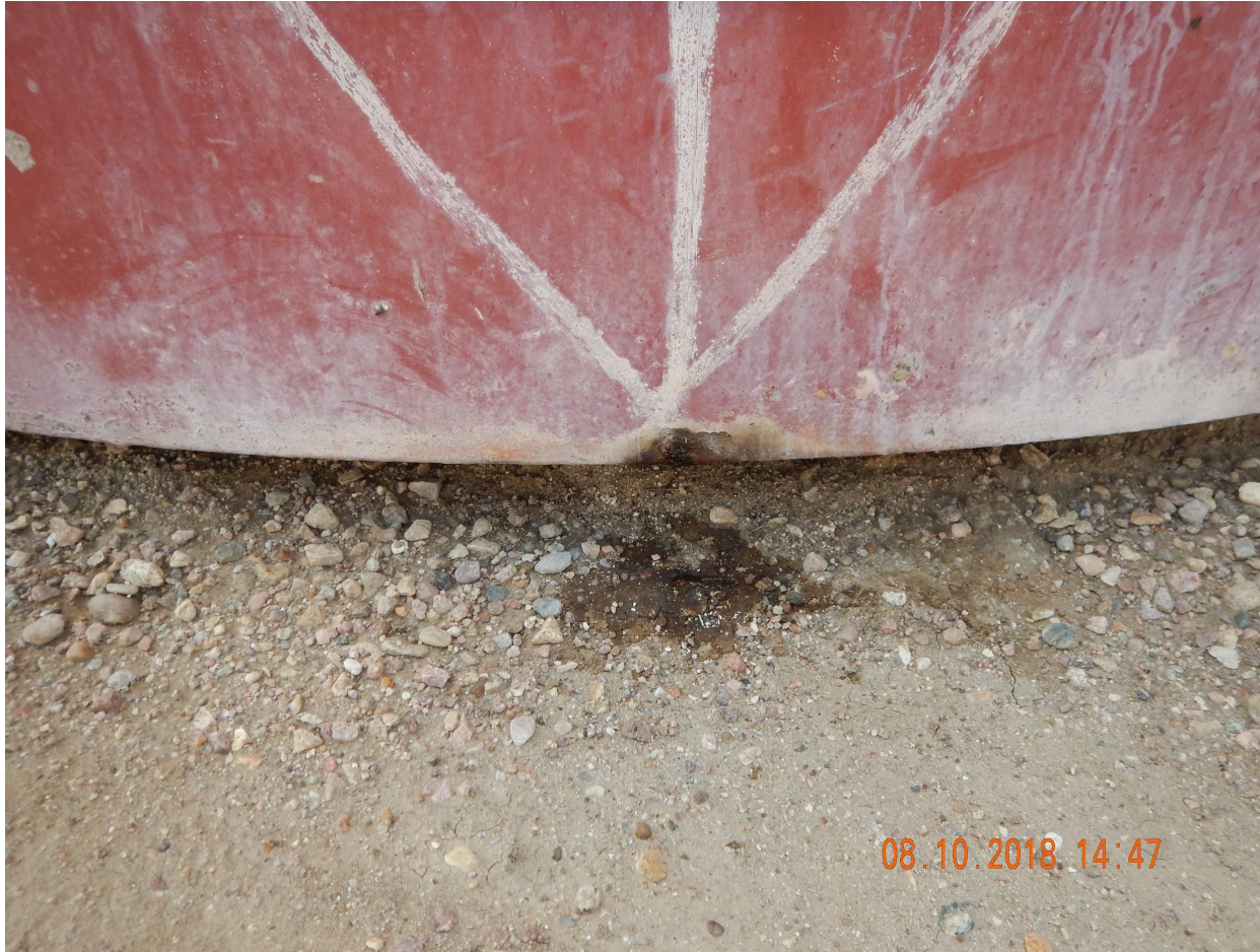
Photo 3. Close up photo taken of the previous tank illustrating a leak needing repair.
