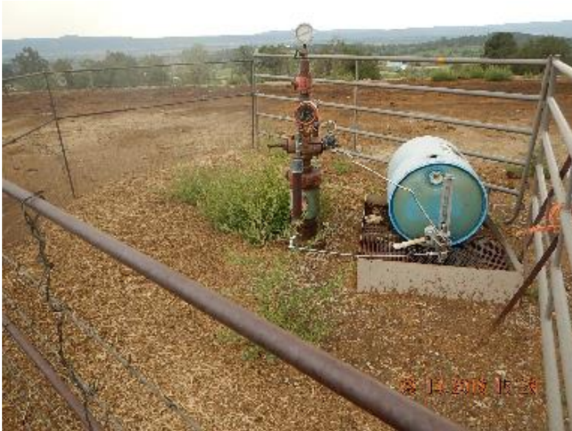
Photo 15: Chemical tank at Argenta 19 missing filler cap.
