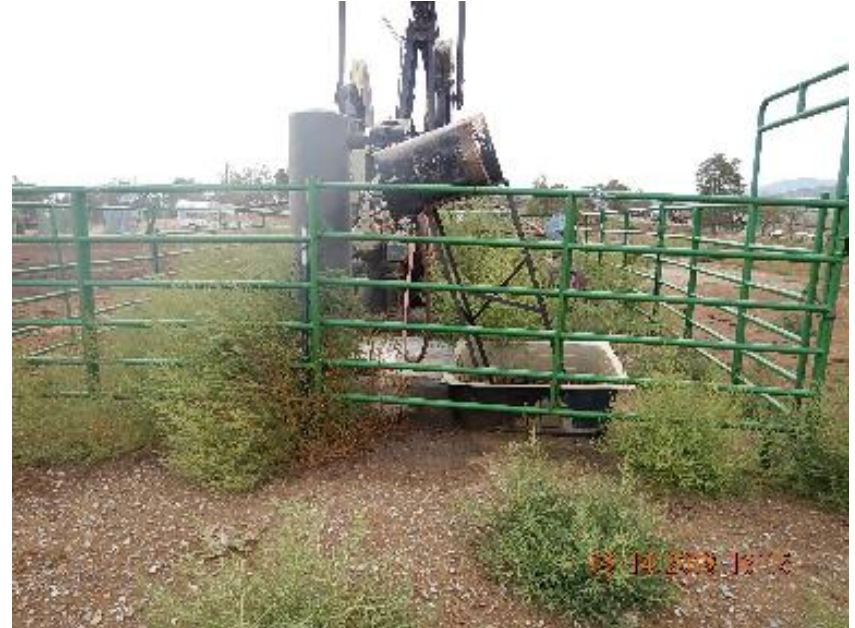
Photo 16: Leaning lube oil tank at the Argenta 18.
