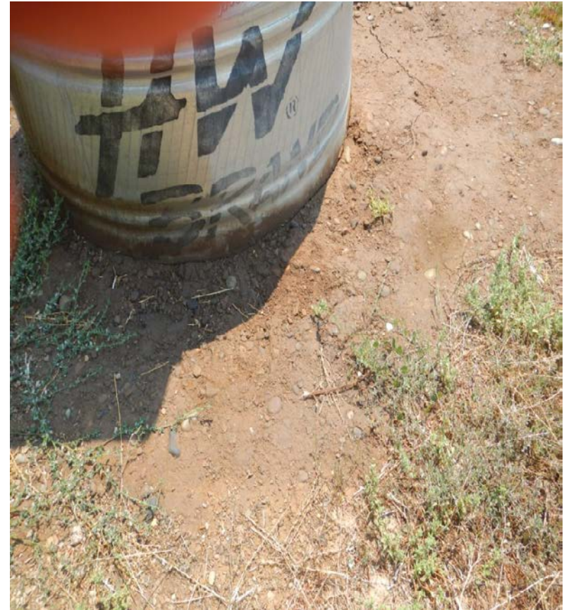
Photo#16: Staining and impacted soil were observed around multiple pieces of equipment.
