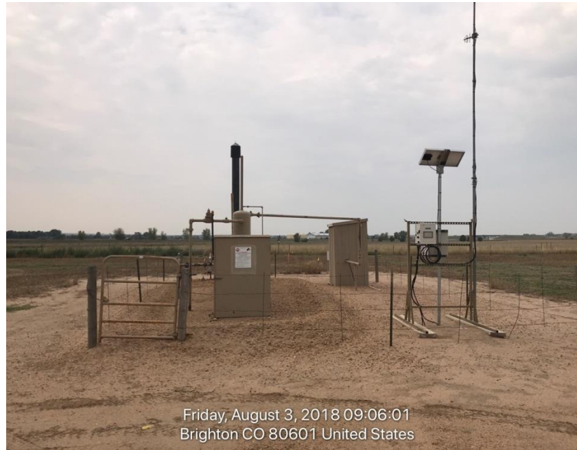
Photo#3 Separator/Gas Meter/Automation RTU
