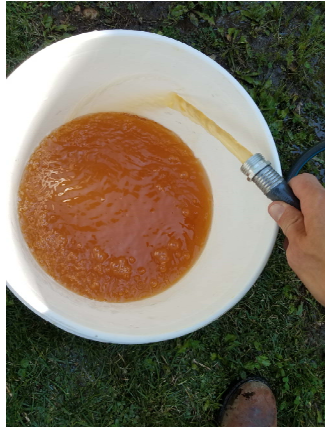
Photo 2 – Purge water showing orange color and turbidity.
