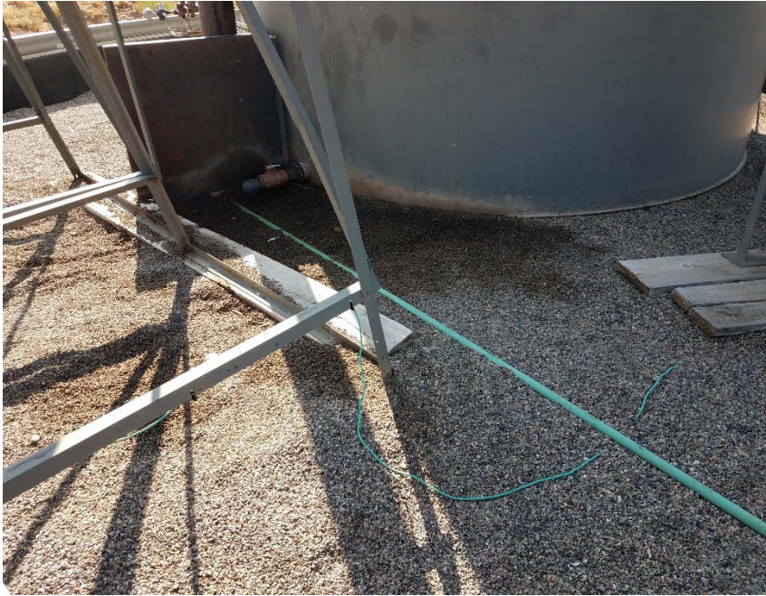
Location Photo #5, Oil stained rock in tank containment.
