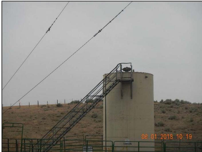
**Photo 3. Gauge hatch open, incorrect emergency contact on signs.**
