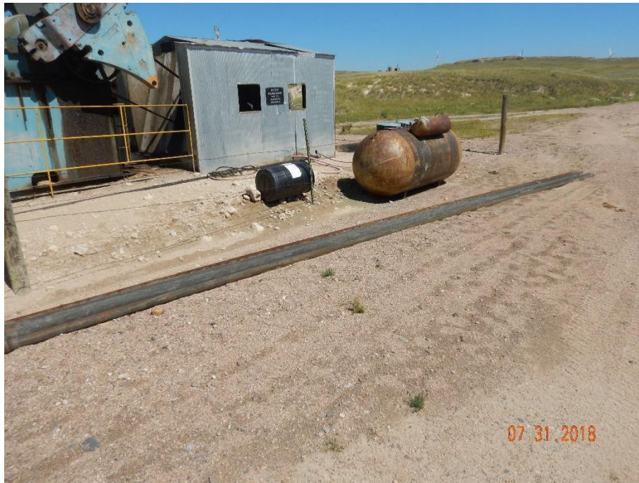
Photo 1: Photo taken from the east end of the location, facing north. Photo shows pipe equipment and barrels laying on the ground. Pipe is unused equipment not needed for production and needs to be removed and properly stored. Barrels need to be placed in secondary containment or removed and properly stored.
