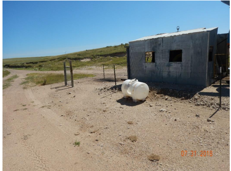
Photo 4: Photo taken from the west end of the location, facing northeast. Photo shows plastic chemical container. Container needs to be placed in secondary containment or removed and properly stored.
