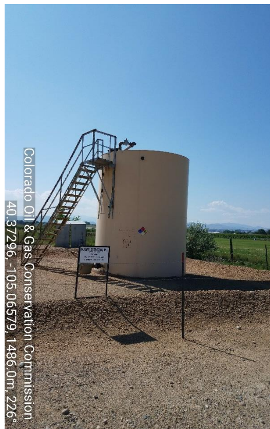
Photo 2 Tank Battery
