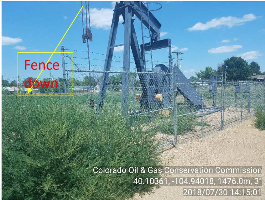
Photo 1. Wellhead Corrective actions: Weeds around wellhead cannot see sign, fence is down on wellhead side of pump jack.
