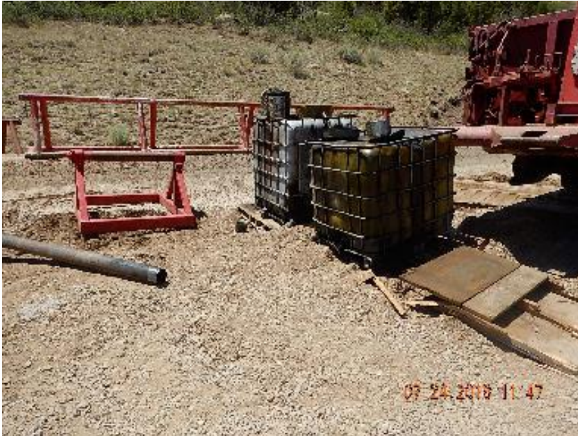
Photo 5: Oil totes with no spill prevention.
