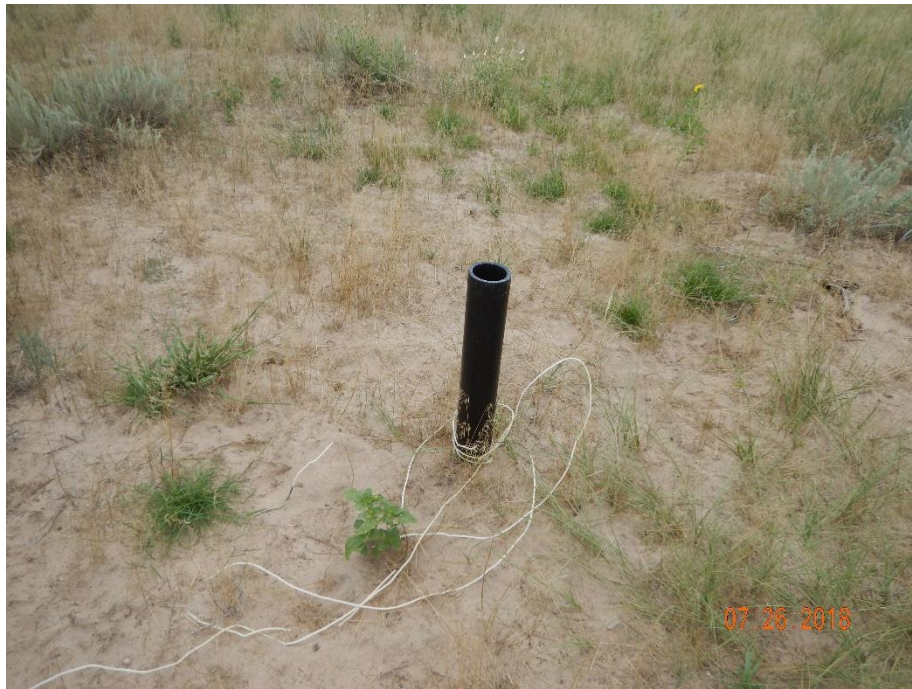
Photo 5: Photo taken from the west end of the location. Photo shows pipe riser remaining on location. Riser needs to be removed in accordance to 1004.a
