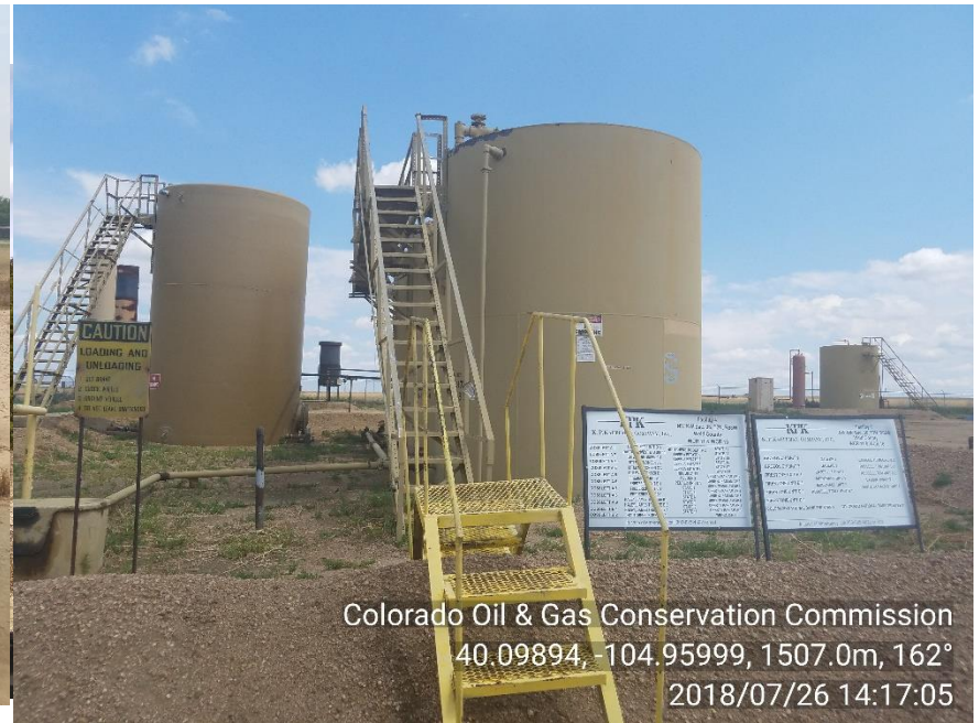
Photo 2. Tank battery
