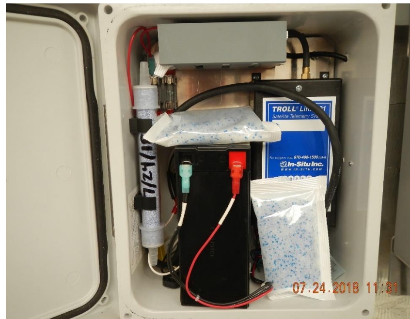
TrollLink 201 equipment enclosure with desiccants replaced.
