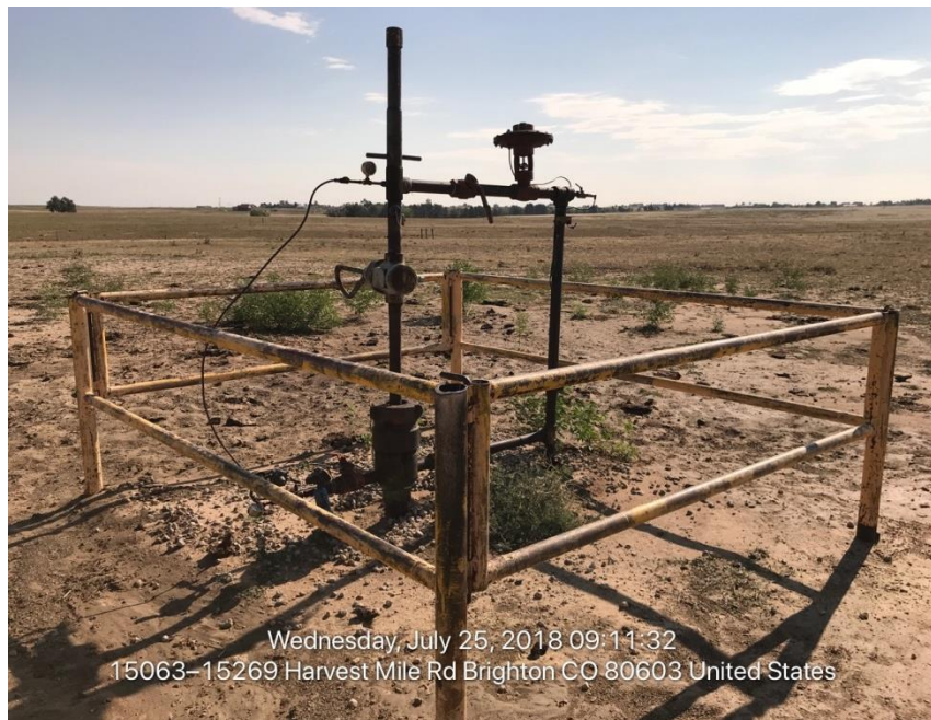
Photo#3 Wellhead/ Wellhead Sign missing
