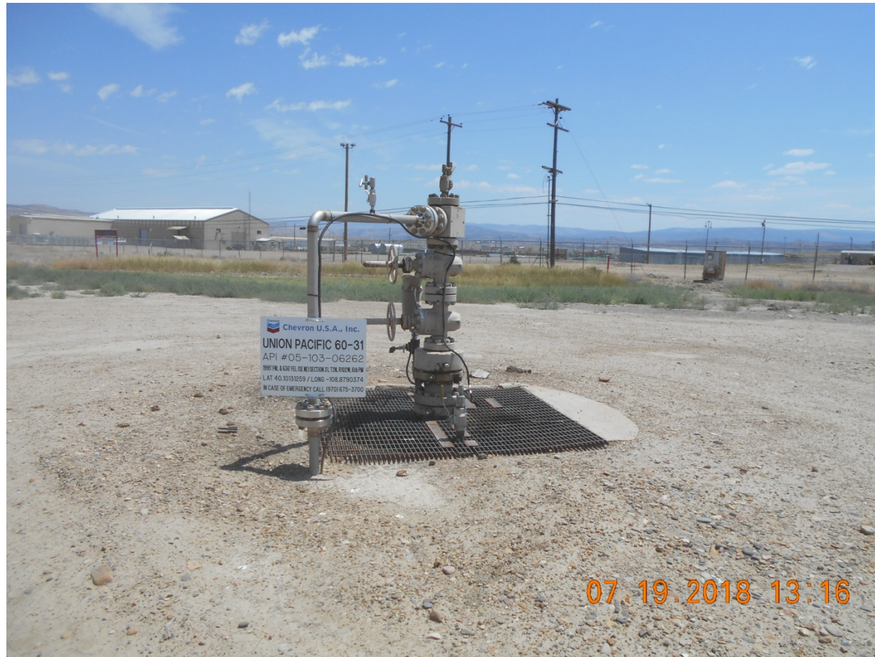
Injection Wellhead
