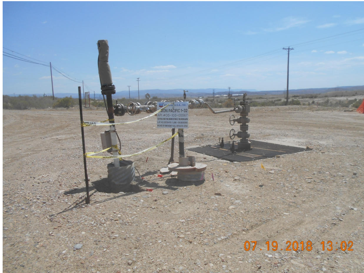
Injection Wellhead
